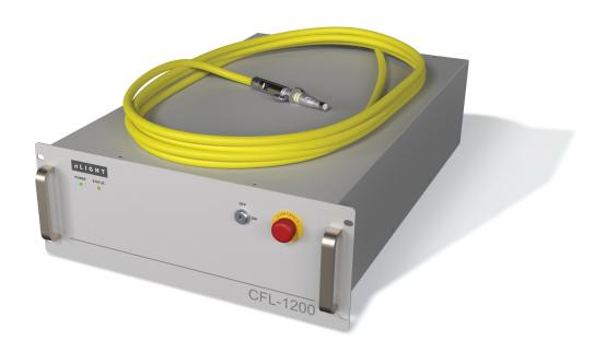
The nLIGHT® single mode rackmount fiber lasers deliver power outputs from 500 to 1200W with beam quality of  $M^2 \le 1.1$  for advanced cutting, welding and additive manufacturing. The small size of these lasers facilitates easy integration into machine tools. nLIGHT rackmount fiber lasers feature true hardware-based back reflection protection, easy onsite servicing and reliable operation in even the harshest manufacturing environments.
