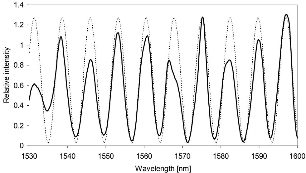
Figure 7. Measured beat spectrum from a 1m long piece of the 30/250 PM-LMA fiber and the sinusoidal fit, giving a birefringence of  $3.1 \cdot 10^{-4} \pm 0.3 \cdot 10^{-4}$ .
