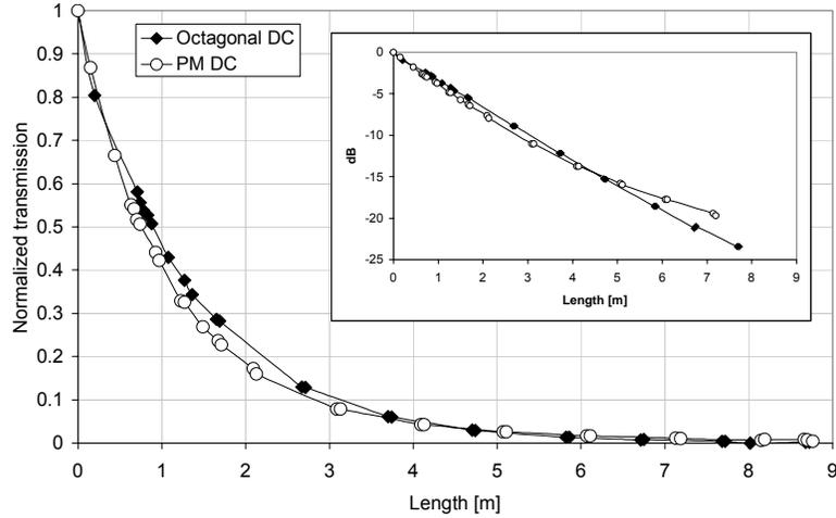
Figure 3. Cladding absorption in octagonal shaped and panda-type PM-LMA double clad fiber versus fiber length.
