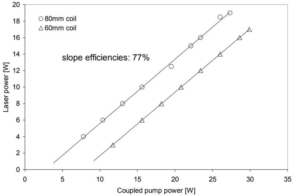
Figure 5. Measured laser output power as the function of coupled pump power for 60mm and 80mm fiber coiling radius.
