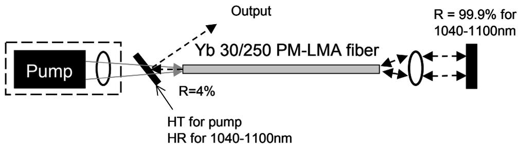
Figure 4. Experimental Yb-fiber laser measurement arrangement. HT: High-transmission, HR: High reflectivity.
