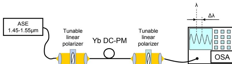
Figure 6. Measurement setup used for the PER and birefringence measurement.
