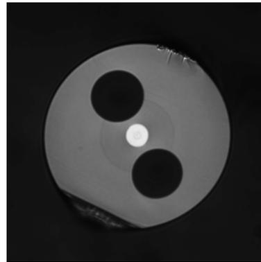
Figure 2. Cross-section of fabricated 30/250 PM-LMA fiber (round cladding deformed in cleaving)
