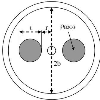
Figure 1. Cross-section of Panda-type PM fiber
