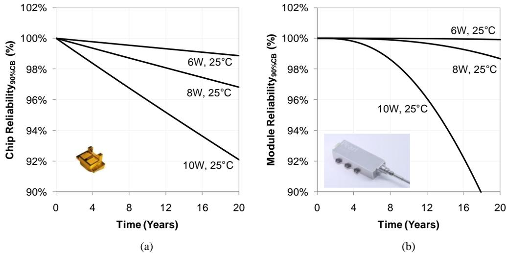
Fig. 7: Reliability (90% lower confidence) vs. time for (a) a single emitter and (b) a 16-emitter module at several emitter power levels. As shown, built-in redundancy leads to lower failure rates early in the life of the module.
