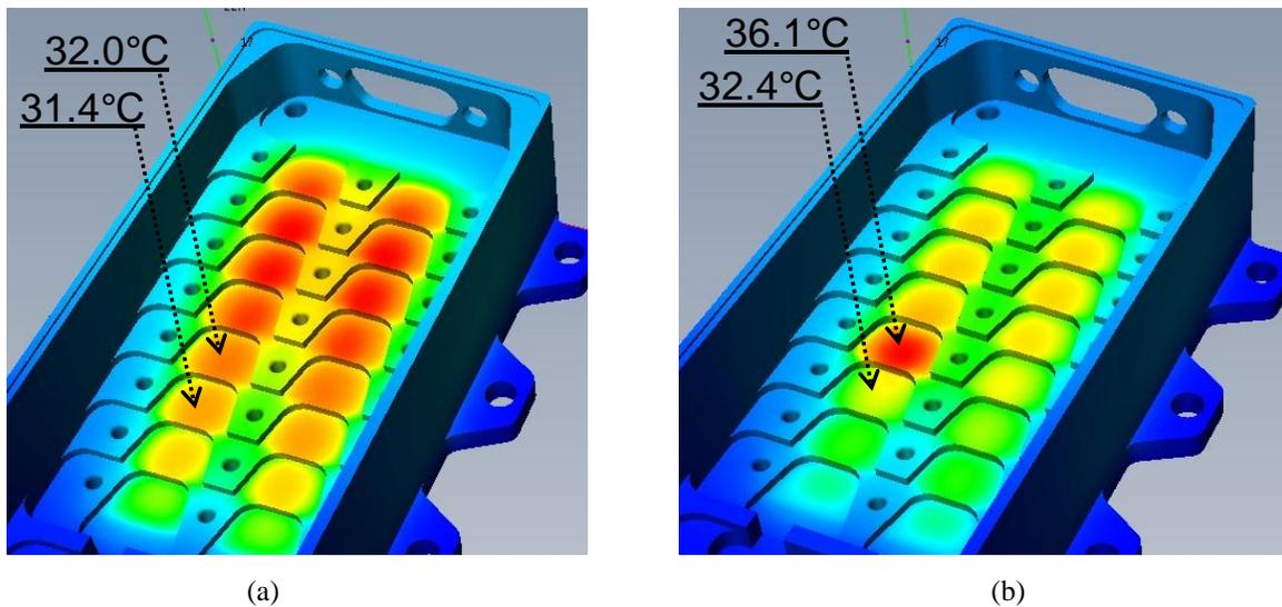
Fig. 5: Finite element thermal analysis of the package heatsink (a) before and (b) after the failure of a single constituent emitter. The failure results in a temperature perturbation of the nearest neighbor of just 1°C
