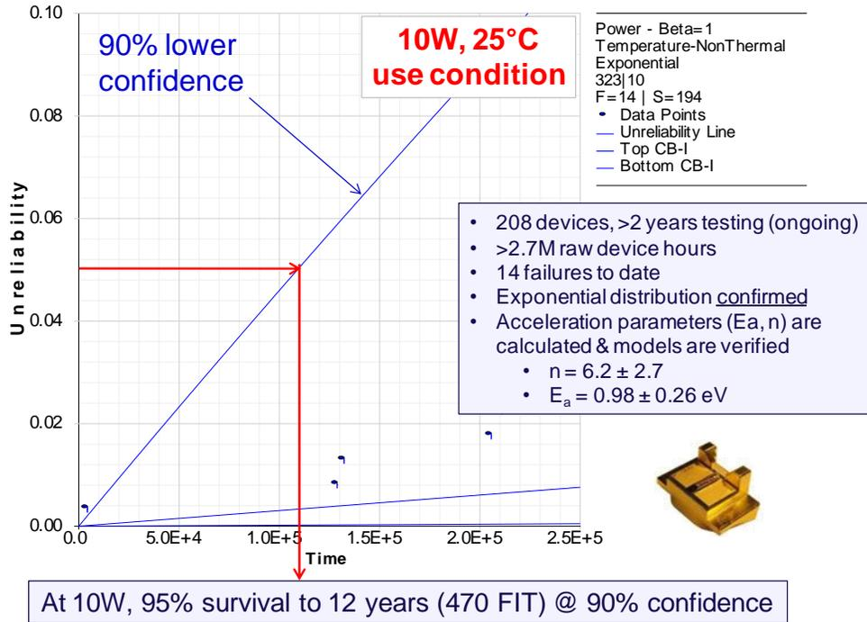
Fig. 2: Summary results of a multicell accelerated lifetest of nLight’s 9xx-nm diodes. At a 10W, 25°C rated use condition, the diodes achieve 95% survival to 12 years @ 90% statistical confidence.
