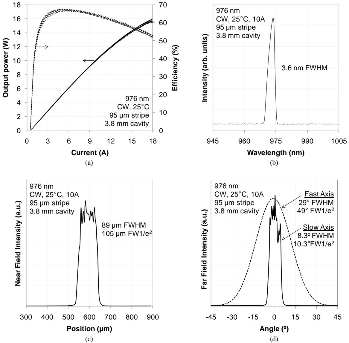
Fig. 1: Typical performance of nLight's 9xx-nm 95  $\mu\text{m}$  stripe single emitter lasers. (a) Power and efficiency vs. drive current for ten devices, measured CW at 25°C. (b) Lasing spectrum, (c) near-field, and (d) far-field intensity profiles measured at 10A.
