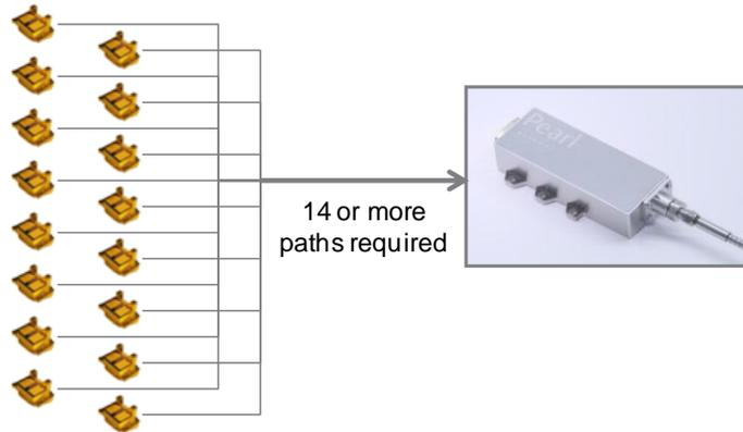
Fig. 6: Block diagram schematic of a 16-emitter module. The reliability of each emitter is considered to be independent of the other emitters. The module is considered to have failed upon the failure of the 3<sup>rd</sup> chip.
