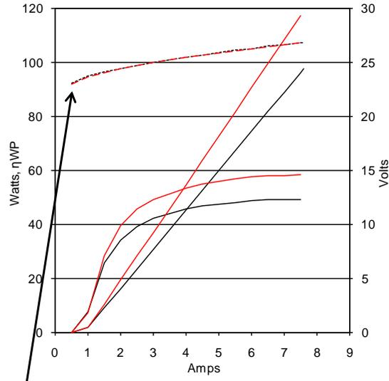
Despite three chip failures, electrical characteristics are unchanged
