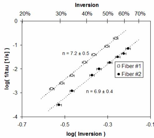
Figure 1. Measured photodarkening rate constant as a function of inversion. The slope of the log-log plot indicates a 7<sup>th</sup> order power dependence.
