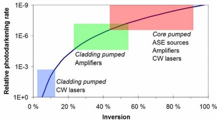
Figure 2. Normalized photodarkening rate as a function of inversion, assuming a 7<sup>th</sup>-order power law. Device application regions with different inversion levels are highlighted.
