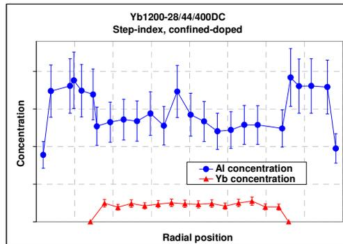
Figure 4. Radial SEM/EDS composition analysis of the core of the Yb1200-28/44/400DC preform. Error bars represent the 95% confidence interval as reported by the measurement equipment.
