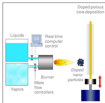
Figure 2. Schematic of Direct Nanoparticle Deposition process for doped silica soot deposition. Both liquid and vapor raw materials can be fed into the burner. The glass is formed in the flame, yielding doped silica nanoparticles that are subsequently deposited on a rotating and traversing mandrel.
