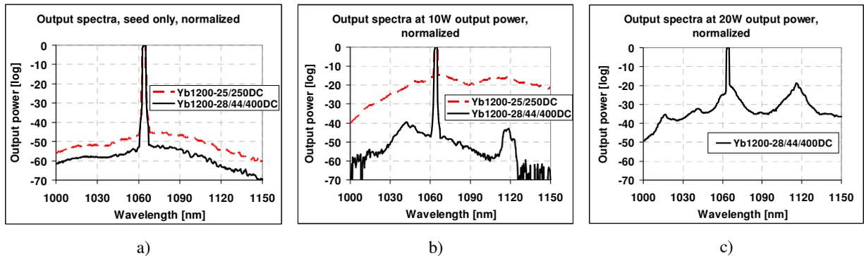
Figure 8. Output spectra of Yb1200-25/250DC and Yb1200-28/44/400DC fibers. a) Seed only b) 10W output power c) 20W output power
