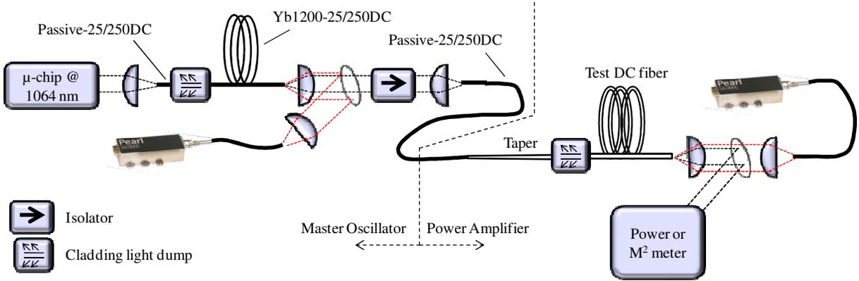
Figure 6. Amplifier setup used to test the fibers.
