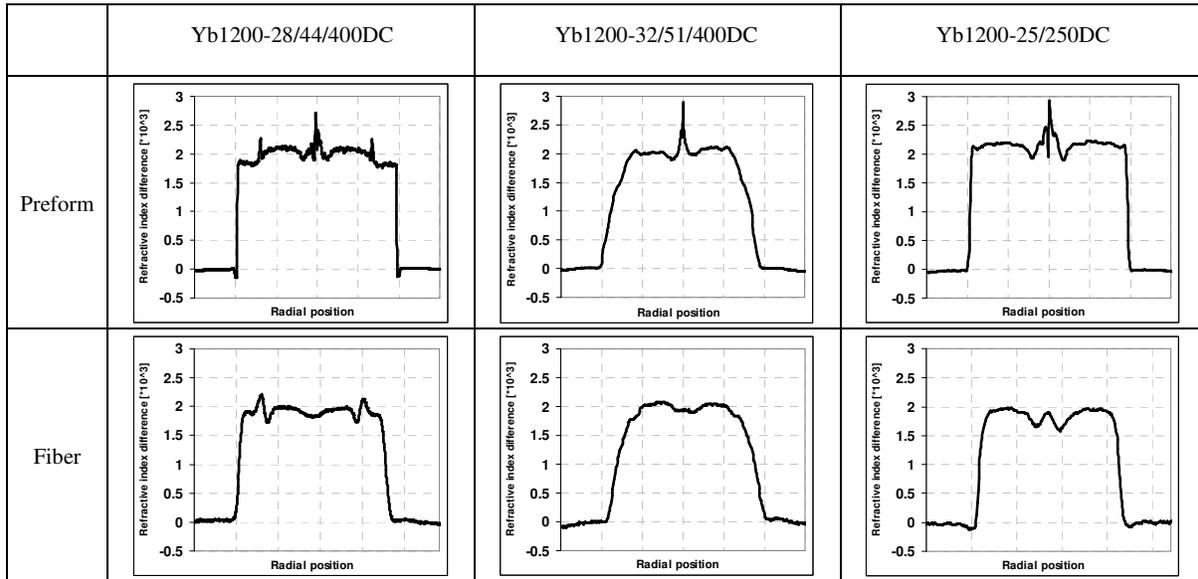
Figure 3. Preform and fiber refractive index profiles of the experimental fibers. The sharp index changes at the material interfaces are attributed to stress related index changes.
