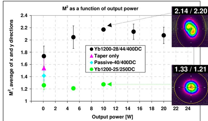
Figure 9. M<sup>2</sup> comparison of conventional Yb1200-25/250DC and confined-doped Yb1200-28/44/400DC. Dots present an average value of M<sup>2</sup>, and the vertical lines indicate the difference in the x- and y-axis direction. Insets show output beam images of both fibers at 10W output power.
