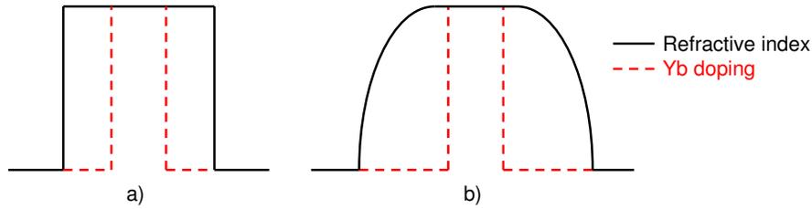
Figure 1. Refractive index and active ion profiles of the new fibers. a) step-index with confined doping b) tailored refractive index with confined doping
