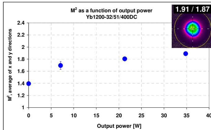
Figure 10. M<sup>2</sup> as a function of output power for the Yb1200-32/51/400DC. Output beam image at 35W shown in the inset.
