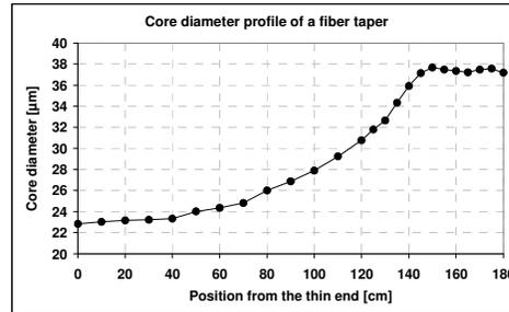
Figure 5. Measured core diameter profile of a typical fiber taper
