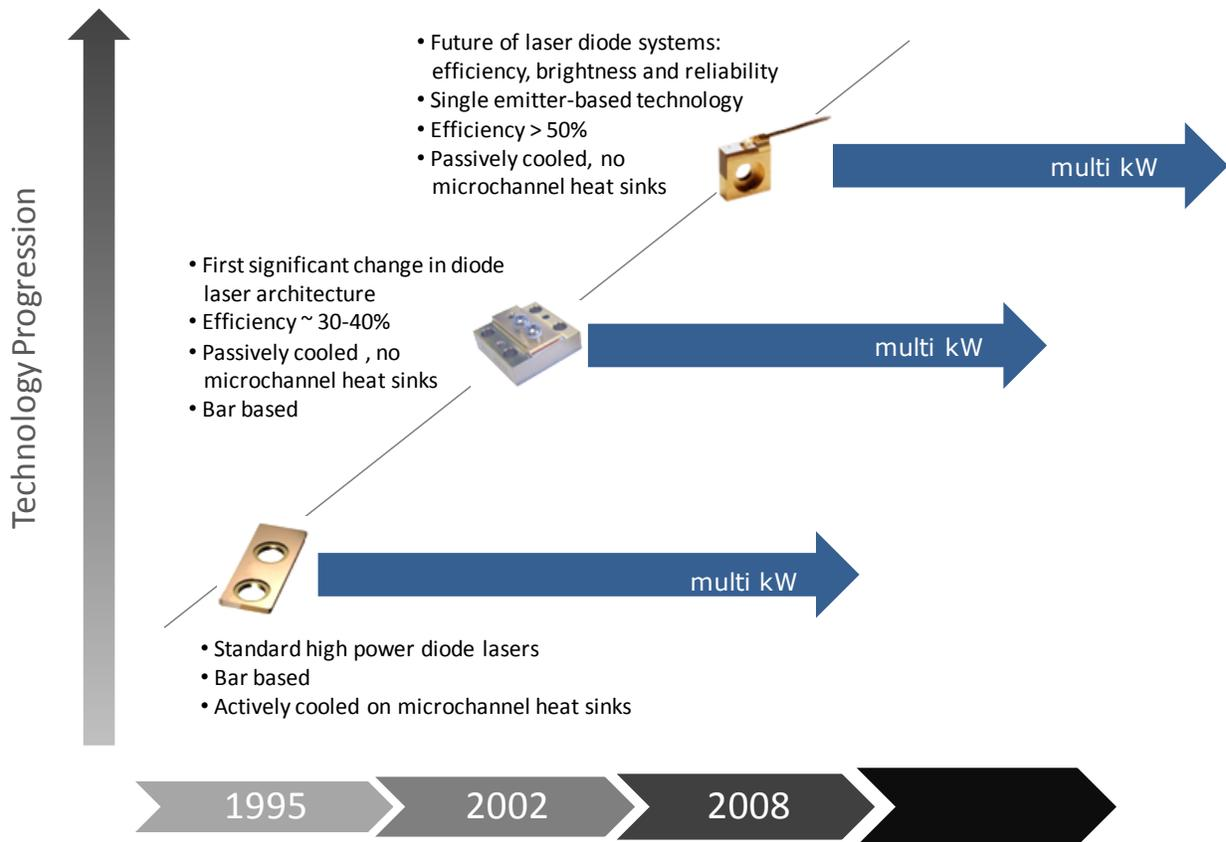
**Figure 4: Technology progression of laser diode systems. The move to single emitter-based diode lasers simultaneously improves brightness and efficiency from the diode laser system.**
