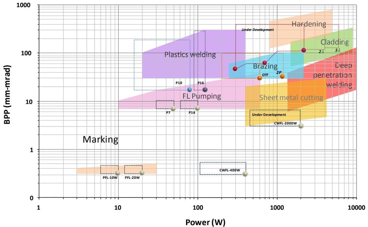
Figure 2: Power and brightness requirements for the industrial laser applications space. Fiber laser and direct diode laser products available from nLIGHT are also shown.
