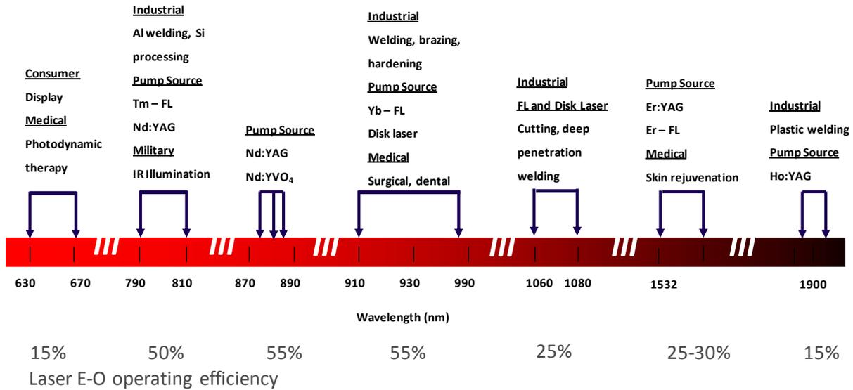
Figure 3: Wavelength requirements for industrial, pumping, medical, and consumer applications with laser electrical-to-optical efficiency.
