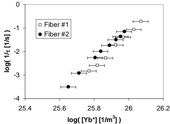
Fig. 9. The same rate data as Fig. 8 re-plotted as a function of excited-state Yb number density  $[Yb^*]$ . The fibers were of similar glass composition and different Yb-ion concentration. The results suggest that the initial PD rate for a given glass composition is determined by the excited-state number density.
