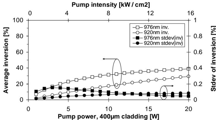
Fig. 4. Average inversion and standard deviation of the inversion vs. pump power for a cladding-pumped, Yb-doped fiber with a  $20 \mu\text{m}$  core diameter and  $400 \mu\text{m}$  cladding diameter. The inversion does not have a practical threshold level after which the inversion is saturated, but rather the inversion is tunable and very flat over a range of pump power. The inversion level is mainly defined by the absorption cross section and the pump power.
