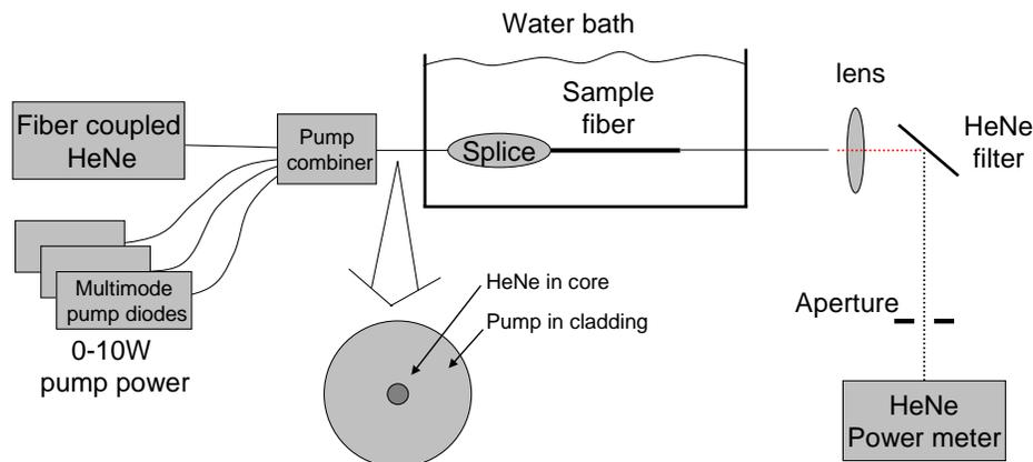
Fig. 5. Measurement setup to measure the PD rate in the Yb-doped core of the sample fiber. A longitudinally constant inversion was achieved with a short sample length, and the inversion level was tuned by varying the pump power. HeNe transmission through the core of the fiber was measured as a function of time as the fiber photodarkened.
