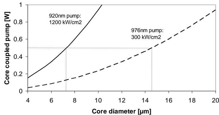
Fig. 3. Maximum saturated core diameter for 920 nm pump wavelength and 0.5 W pump power is approximately 7 µm presuming the 1200kW/cm<sup>2</sup> requirement for pump irradiance. For 976 nm pumping, the irradiance of 300 kW/cm<sup>2</sup> is reached at approximately 14 µm when using 0.5 W of pump power.
