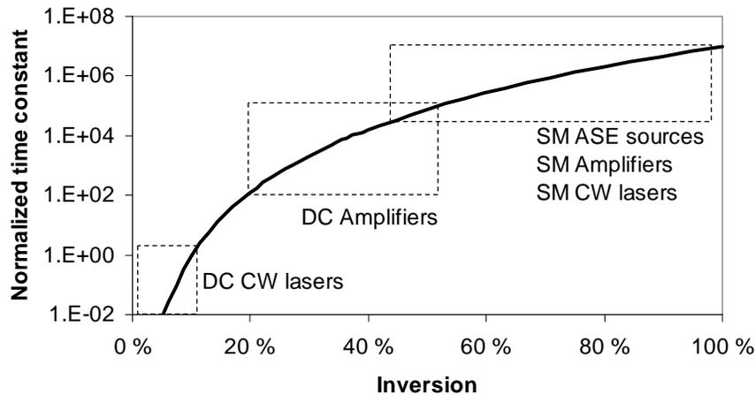
Fig. 10. The normalized initial PD time constant as a function of inversion, presuming a seventh-order dependence on inversion. Operating regimes for various applications are highlighted.
