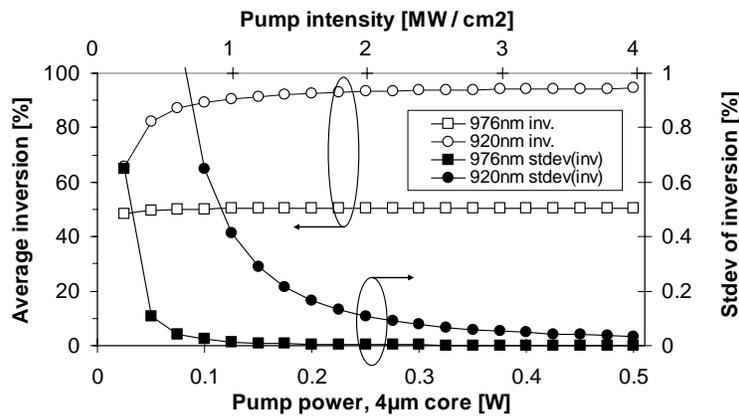
Fig. 2. Average inversion and standard deviation of the inversion vs. pump power for a core-pumped, Yb-doped fiber. The inversion of the sample saturates, i.e. additional pump power no longer increases the inversion. The saturated inversion level is mainly defined by the ratio of absorption and emission cross sections.
