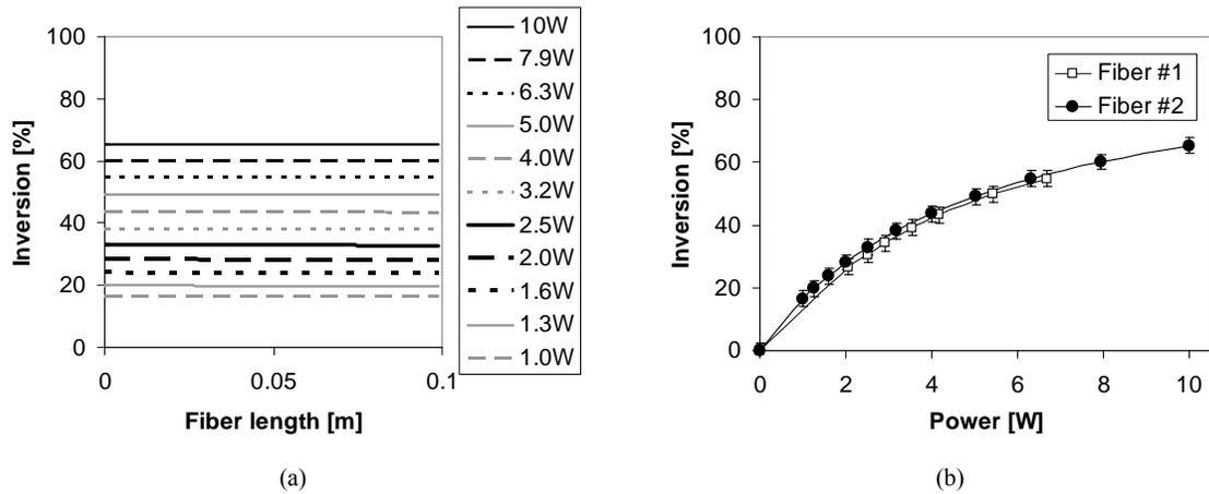
Fig. 6. (a) Longitudinal inversion profile of short (10 cm) sample fibers cladding pumped using different pump powers. The induced inversion profile is spatially very flat and tunable over a wide range. (b) Simulated average inversion of fiber samples as a function of pump power.
