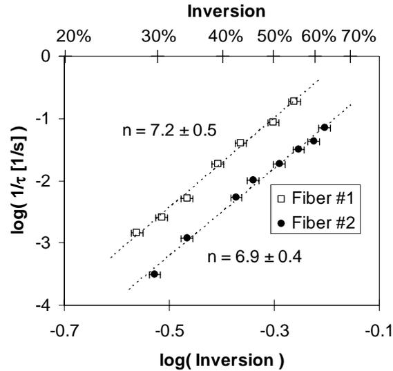
Fig. 8. Log-log plot of the inverse of the PD time constant as a function of inversion. The data for both fibers are well described by a linear fit with a slope of  $\sim 7$ .
