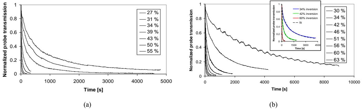
Fig. 7. (a) Measurement results of Fiber #1. (b) Measurement results for Fiber #2. The probe transmission at different inversion levels are shown in the same order as indicated in the legend, lower inversion as slowest. The inset figure has examples of the fit data together with the measured data.
