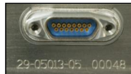
Low-current 15-pin, micro-D connector for data & current
