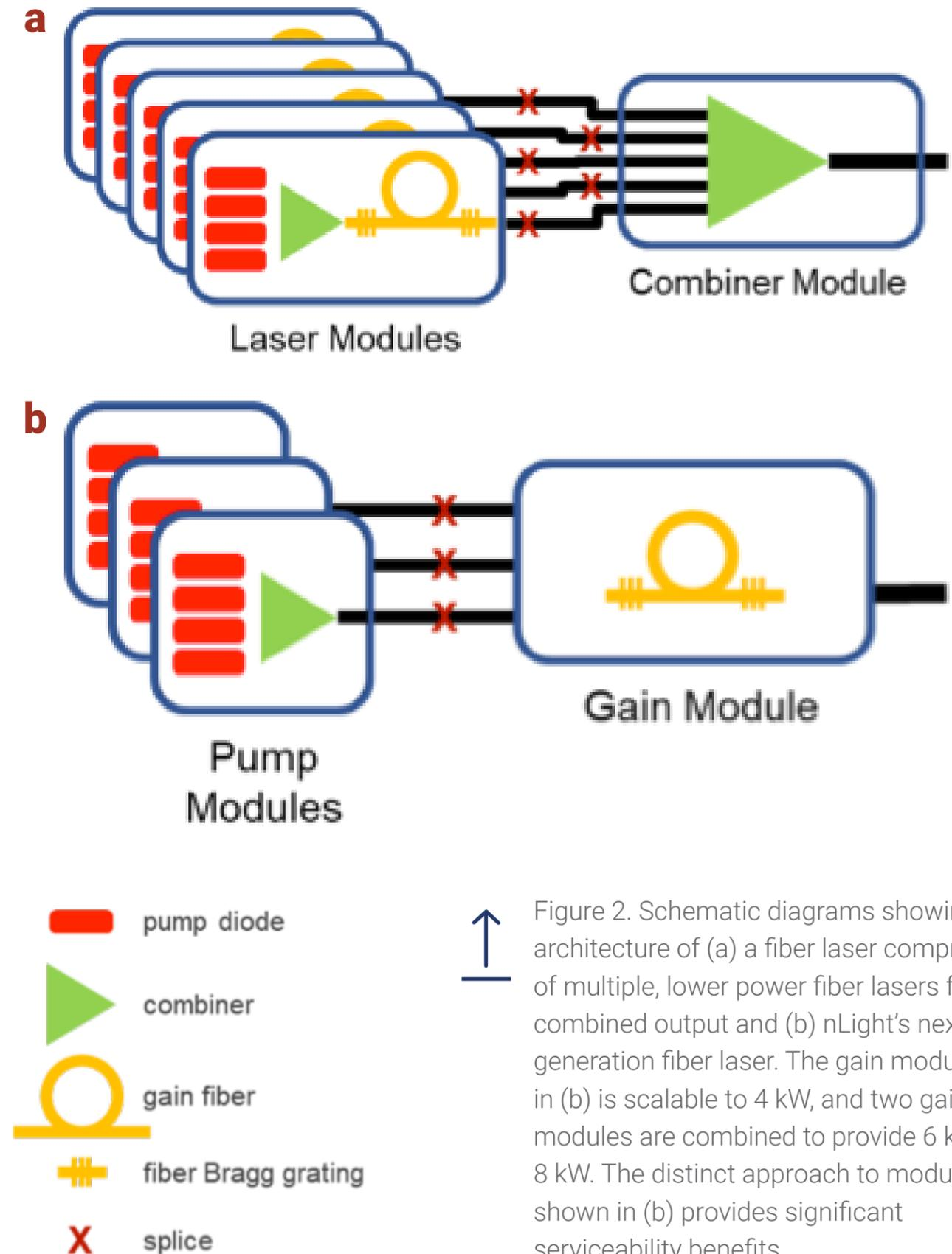
↑ Figure 2. Schematic diagrams showing the architecture of (a) a fiber laser comprised of multiple, lower power fiber lasers for combined output and (b) nLight's next-generation fiber laser. The gain module in (b) is scalable to 4 kW, and two gain modules are combined to provide 6 kW to 8 kW. The distinct approach to modularity shown in (b) provides significant serviceability benefits.
